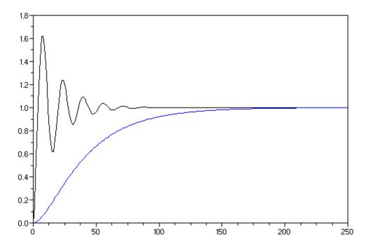
H1's step response (in black) rings like a bell, due to the underdamped nature of the system. H2 is very overdamped, and while it takes much longer to respond it never overshoots.
