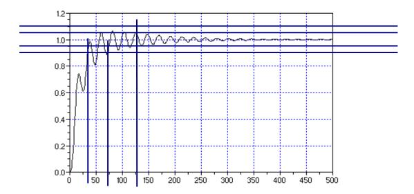
It is impossible to be precise. The four horizontal traces are placed at approximately 90%, 95%, 105% and 110% of the final value; the points where the trace intersects with these lines will be our critical times.
